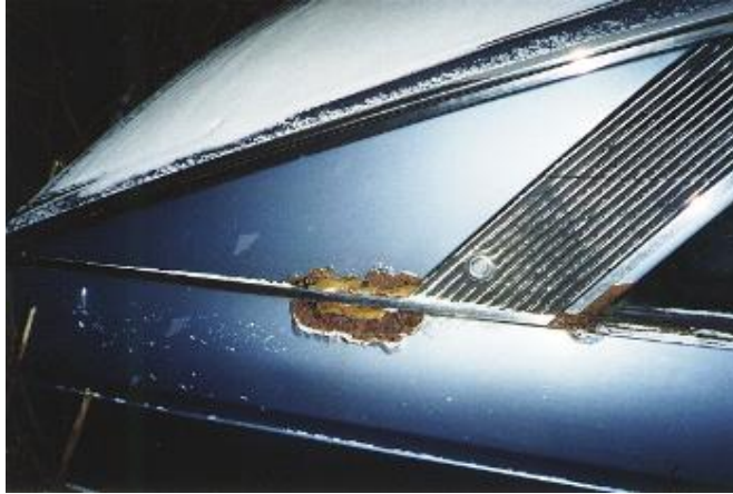
Figure 4.: Rusted out car.
